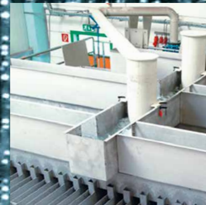
Testing of a trough-type distributor
