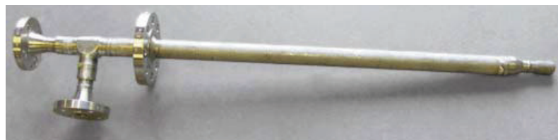
Steam-jacketed fabrication with three spray nozzles installed through the jacket.
